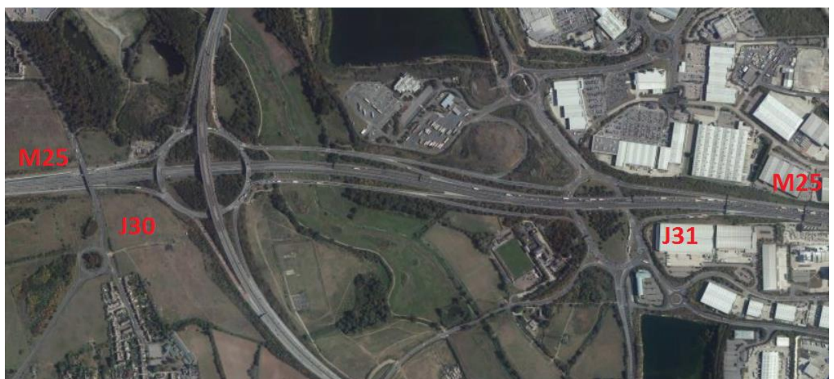
Example of parallel slip roads – J30 to J31 on M25. Traffic from the J31 roundabout has to pass through J30 to access the M25 northbound. However, traffic from the south (right) on the mainline M25 can access both junctions 30 and 31 directly (credit: Bing Maps ©)
