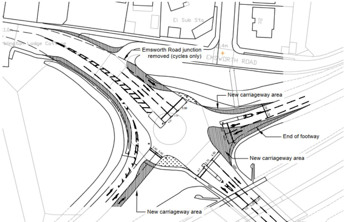
Figure 6.6: Proposed Northern Roundabout (Warblington Interchange) Layout
