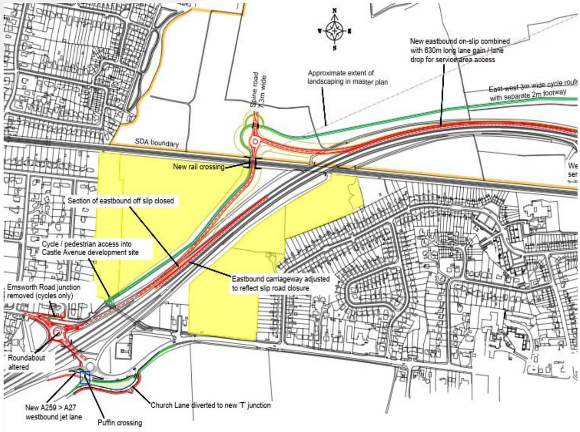
Warblington interchange proposed option 1B – further detail on the potential jet lane arrangement
