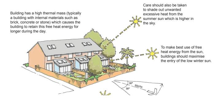
4.41 Active Solar Gain - building facades and roofs can be used to collect solar energy for conversion into electricity or to heat water for the building's occupants. An aspect within 30 degrees due south is ideal.
