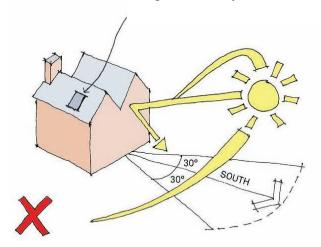
PV / solar water panel facing 30 degrees of south maximises the movement of the sun.
