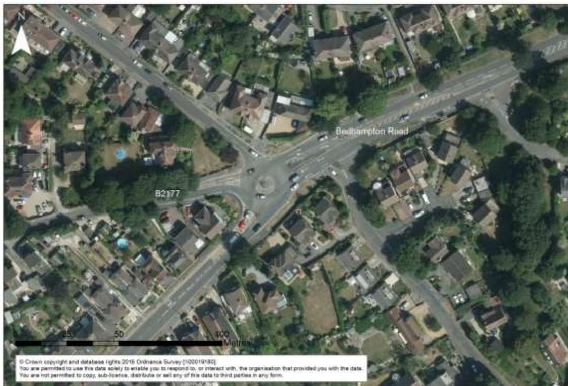
6.1.15. Drawing EC/RJ506423/104 attached in Appendix N of the SRTM Modelling Report shows that mitigation at Junction ID10 primarily involves converting the mini-roundabout junction to a fully signalised junction, with local kerb realignment and widening on the Bedhampton Hill and Maylands Road approach. This also enables improvements to the pedestrian infrastructure by introducing a full signalised
