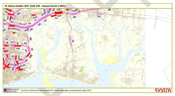
Figure 6-16 Volume Over Capacity - Do Minimum 2036 (PM)
