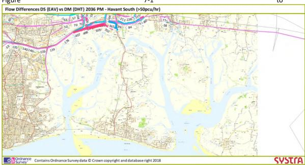
7.3.4 Figure 7-4 show the change in traffic flow in the AM and PM peak hours between the Do Something and Do Minimum scenarios in 2036, at an overall Borough level (Appendix I
