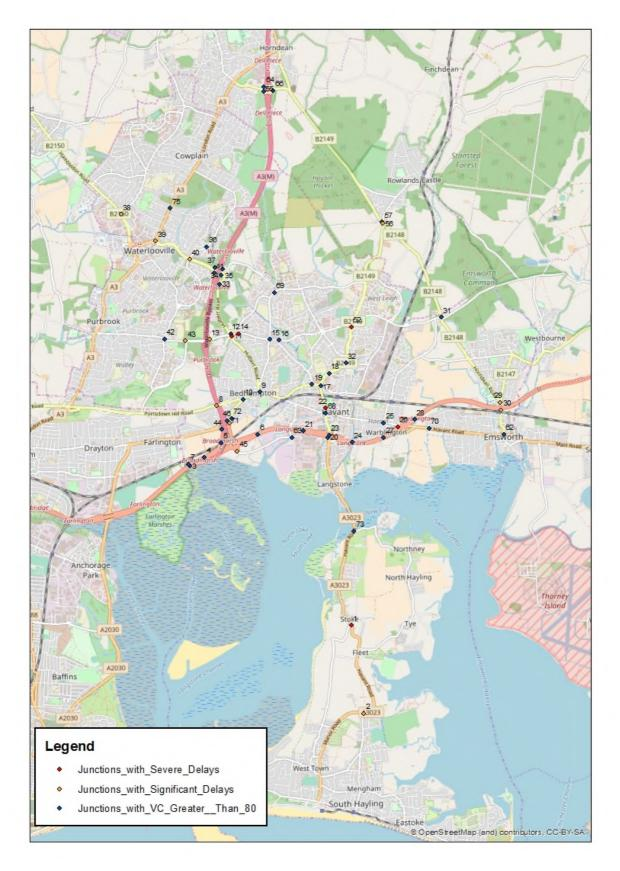
Figure 6-17 Junctions forecast to meet the 'significant' or 'severe' criteria or V/C >80%
