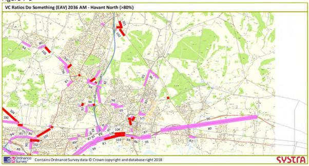
7.3.28 Figure 7-9 to Figure 7-12 display the V/Cs for the AM and PM peak hours for the Do Something scenario (more localised plots are provided Appendix K). For the V/C plots the performance of the link is identified through the colour of the link as follows:
