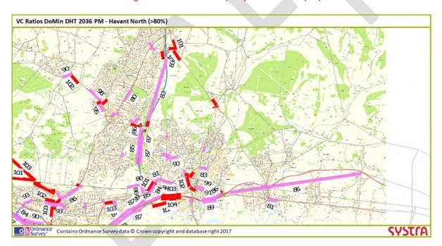
Figure 6-14 Volume Over Capacity – Do Minimum 2036 (PM)
