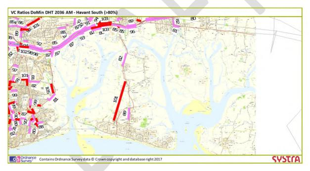
Figure 6-12 Volume Over Capacity – Do Minimum 2036 (AM)
