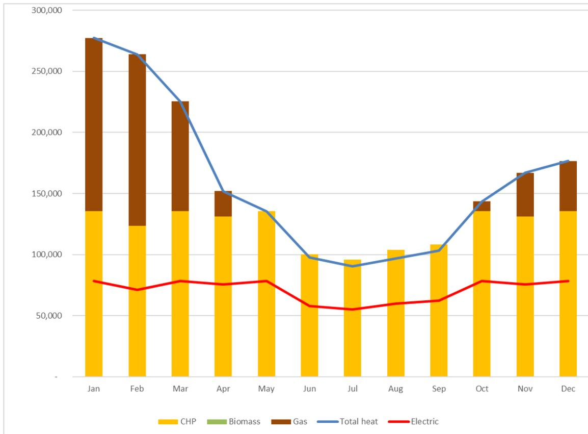
Figure 5.4 Heat supply profile for Havant Heat Network by fuel type – Phase 1 only (165kWe CHP only, 5148 hrs @ 90% availability)
