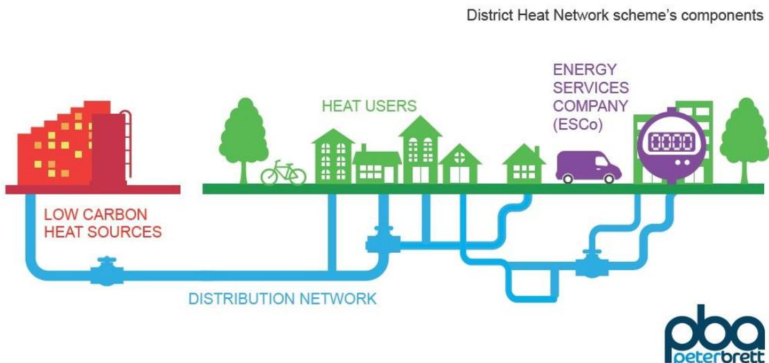
Figure 1.2 Principal infrastructure of a heat network
