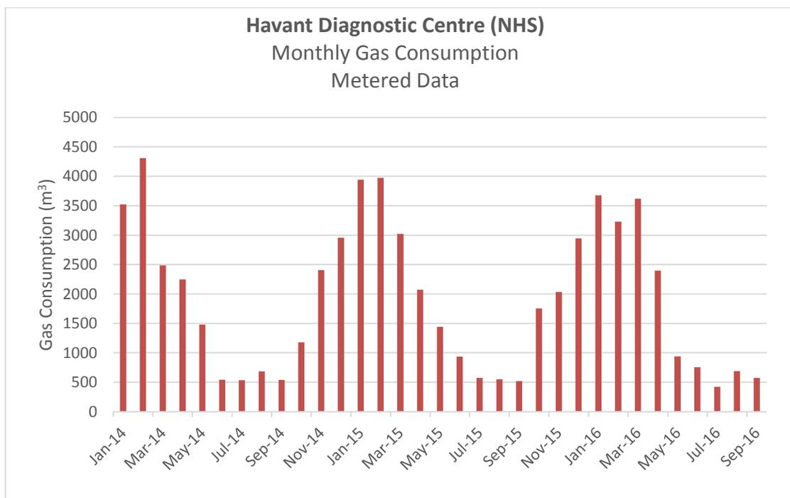
Figure 3.14 – Havant Diagnostic Centre Gas Consumption
