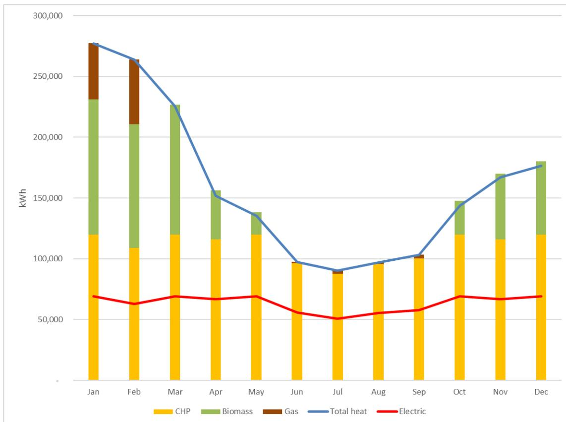
Figure 5.2 Heat supply profile for Havant Heat Network by fuel type – Phase 1 only (165kW CHP, 150kW biomass)
