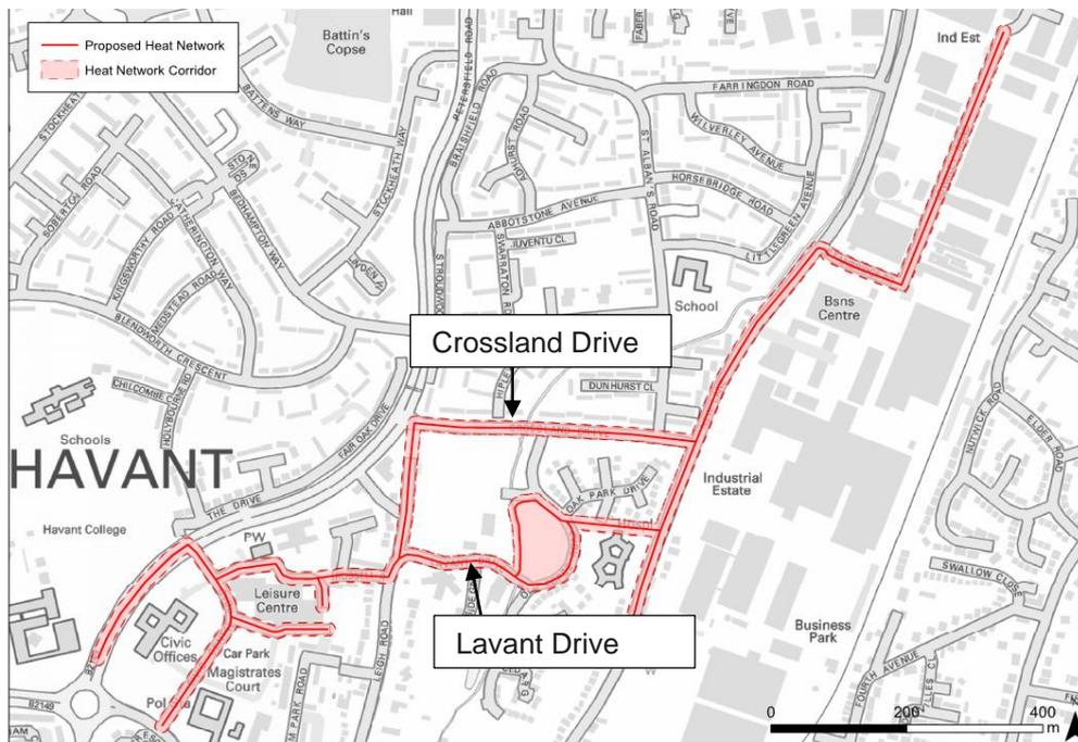
Figure 6.1 Proposed heat network routing for utility search<sup>24</sup>
