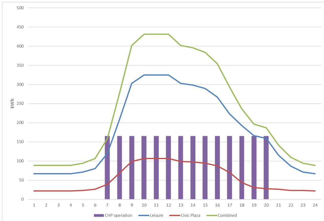
Figure 5.3 Typical daily electrical demand profiles for Civic Plaza and Leisure Centre compared to CHP electrical generation (165kWe, 14hrs)
