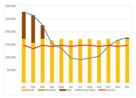
Figure 5.6 Heat supply profile for Havant Heat Network by fuel type – Phase 1 only (310kWe CHP only, 5,588 hrs @ 90% availability)
