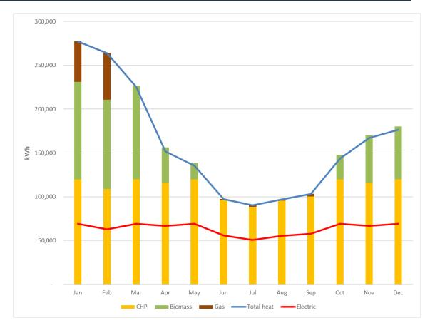
Figure 5.2 Heat supply profile for Havant Heat Network by fuel type - Phase 1 only (165kWe CHP, 150kW biomass)
