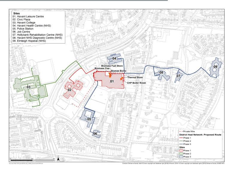
Figure 6.3 Proposed primary network design- Civic Campus (an Interactive PDF of this scheme design is shown in **Appendix E**) (Contains Ordnance Survey data (c) Crown copyright and database right 2016. (c) Crown copyright and database rights 2016. Ordnance Survey 0100031673.)
