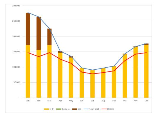
Figure 5.5 Heat supply profile for Havant Heat Network by fuel type – Phase 1 only (310kWe CHP only, 4,542 hrs @ 90% availability)
