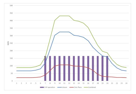
Figure 5.3 Typical daily electrical demand profiles for Civic Plaza and Leisure Centre compared to CHP electrical generation (165kWe, 14hrs)
